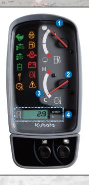
**1** Fuel level gauge **2** Water temperature gauge
